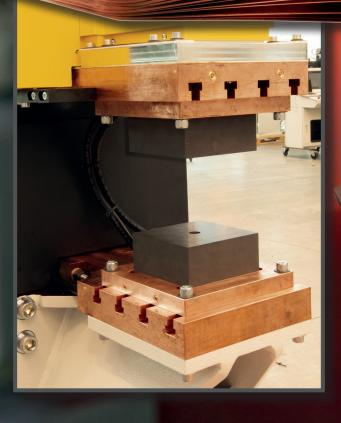
From open linear press to large portal frames, up to 900x600 mm effective area, 40 tons of force and 800kVA of power
